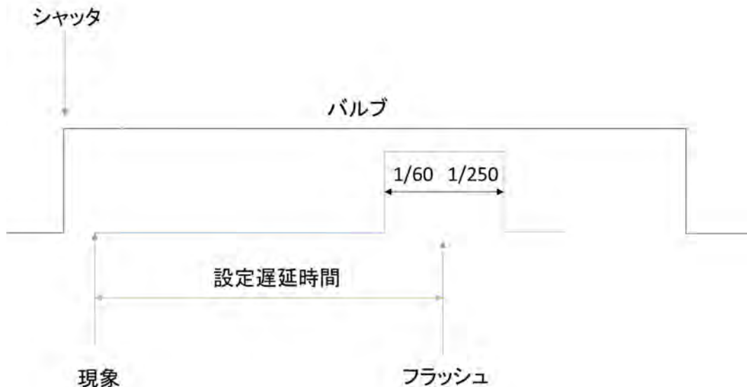
Fig.5 Timing Diagram of Event and Flash lighting relation
