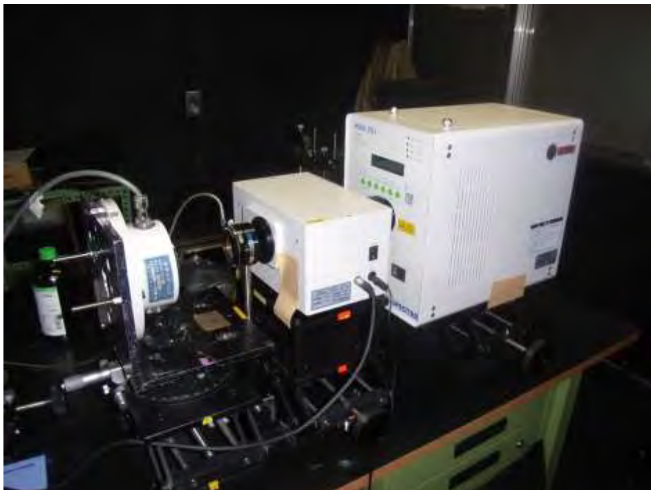
Figure 3 Photograph of a spectral response measurement of solar UV-B irradiance meter used with the calibration and spectral response measurement system developed.
