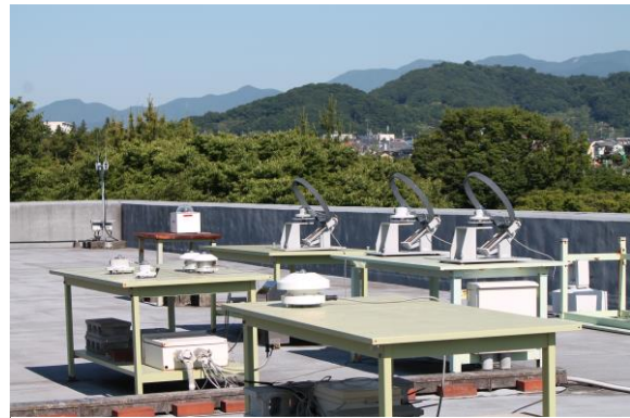
Figure 1 Photograph of solar radiation monitoring system installed at the Shonan Campus of Tokai University.
